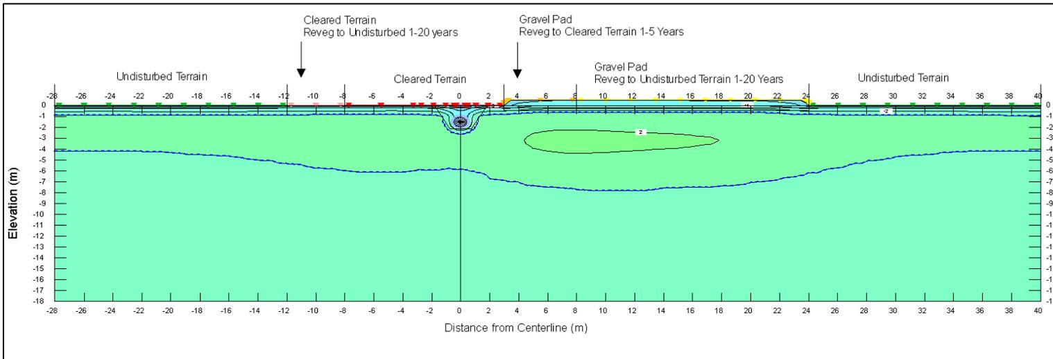
**Figure 4 ROW 30-Year Thaw Depth Profile for Case without Buried Organic Layer below Gravel Pad, 0.08 °F/yr Climate Warming**
